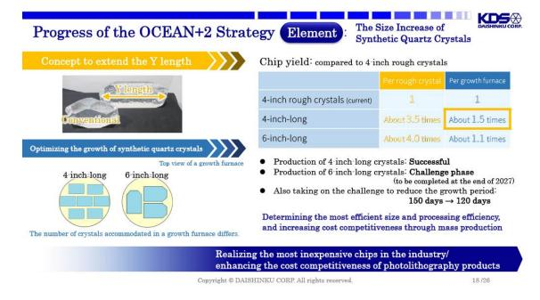
"E" stands for "Element: The Size Increase of Synthetic Quartz Crystals." We have previously discussed the development of larger artificial crystals in 4-inch, 6-inch, and 8-inch sizes. Currently, 8-inch seed crystals are growing as planned. As a trial initiative at the growth stage, we have successfully grown 4-inch long raw crystals.
