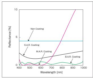
\*Reflectance characteristic per one side (reflectance of back side is not included) .
