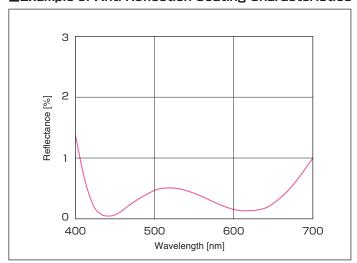
\* Reflectance characteristic per one side (reflectance of back side is not included).
