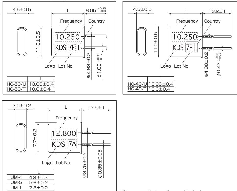
\*Measurement between the root of the leads.
