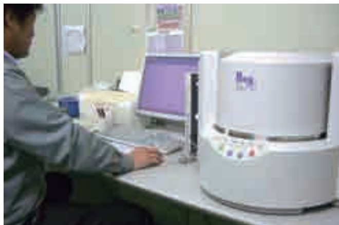
X-ray fluorescence analyzer(Quality Assurance Div.)
